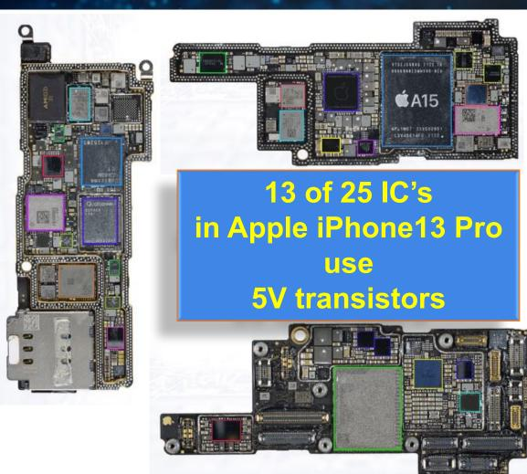
Apple APL1W07 A15 Bionic PoP (A15 AP + SK hynix 6GB LPDDR4X SDRAM) Apple APL1098 PMIC NXP Display Port Multiplexer Skyworks SKY58271-19 Front-End Module Skyworks SKY58270-17 Front-End Module Apple/Dialog Semi 338S00770-B0 PMIC Apple/Dialog Semi 338S00762-A1 PMIC STMicroelectronics STB601A05 PMIC USI Apple U1 UWB Module Texas Instruments TPS65657B0 Display Power Supply KIOXIA 256 GB NAND Flash Apple/Cirrus Logic Audio Codec
